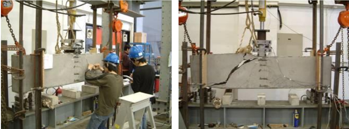
Figure 10.10 Typical share failure mode
