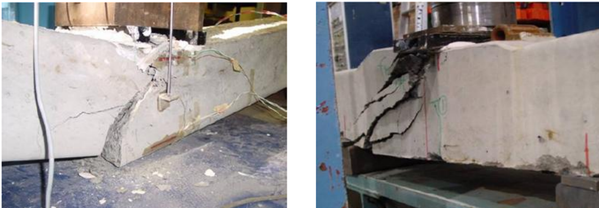
Figure 1.2 Railway concrete sleepers under impact loadings (pictures taken from Remennikov & Kaewunruen, 2007 )
