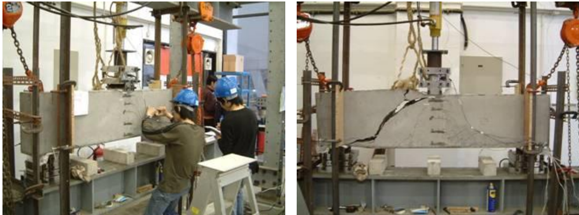
Figure 10.10 Typical share failure mode
