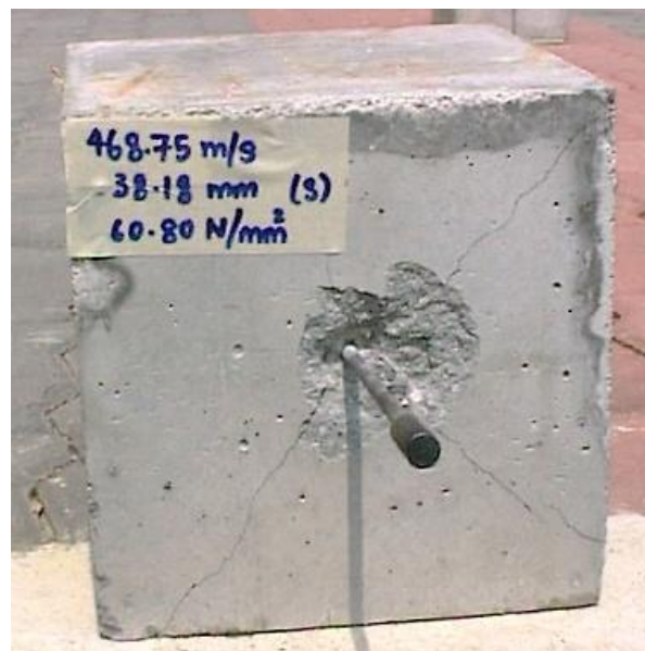
Figure 1.3 Impact of steel nail into concrete a block
