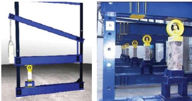
Figure 3.8 Devices for uniaxial creep tests (Tomanović, 2009)
