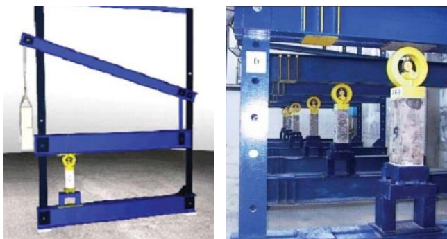
Figure 3.8 Devices for uniaxial creep tests (Tomanović, 2009)
