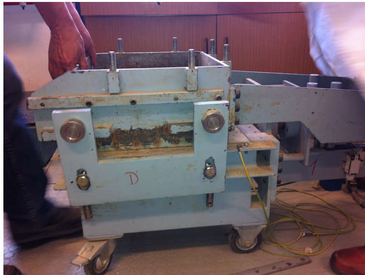
FIGURE 4.8: Large direct shear box at CEI
