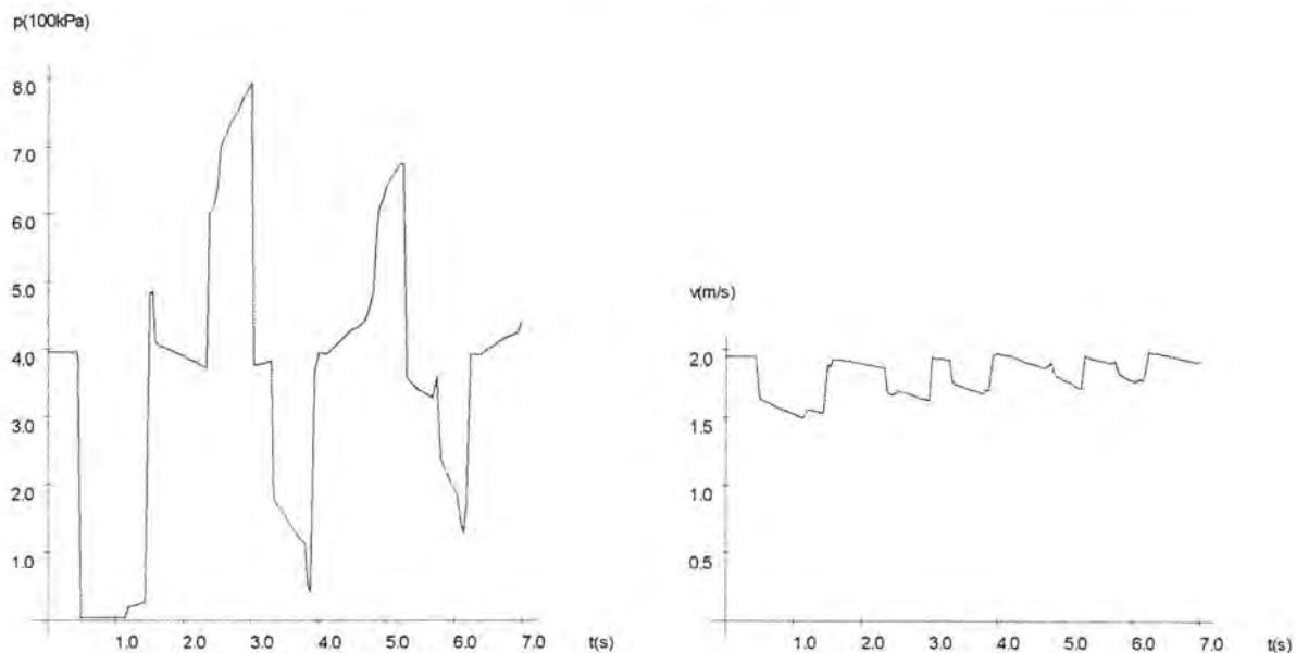
Sl. 48.iii) Proračun 3.5 – tlak i brzina kod  $x = 597\text{m}$
