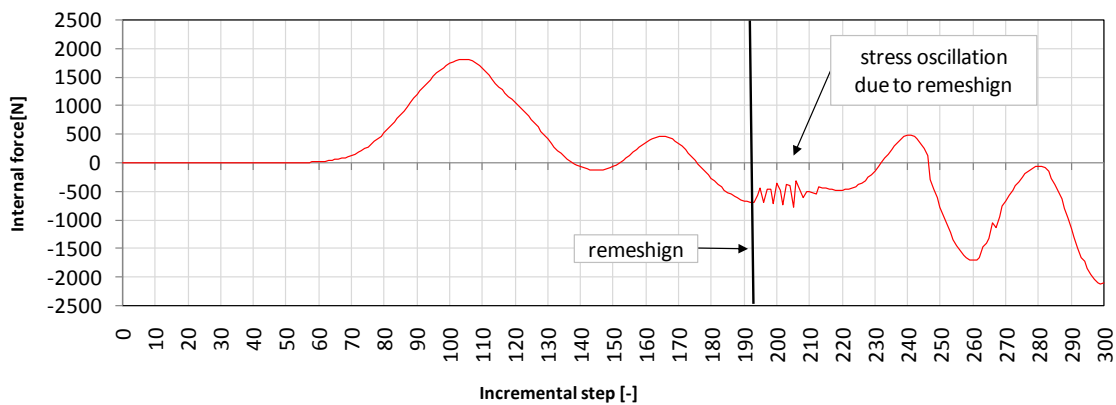
Figure 10.24 Oscillation of stresses after remeshing (after few time increments the oscillations disappear)
