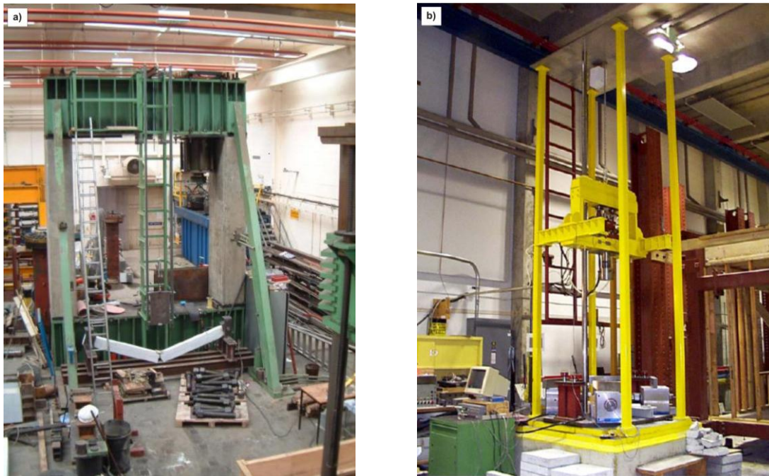
Figure 1.1 Free fall drop weight test. Pictures taken from: a) May et al. (2005) and b) Sukontasukkul et al. (2004)
