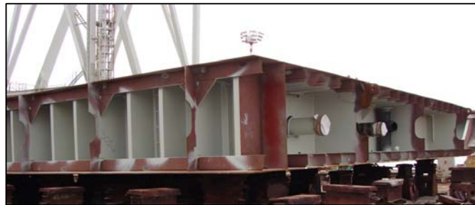
Fig. 3.54. Typical double bottom block [29]
