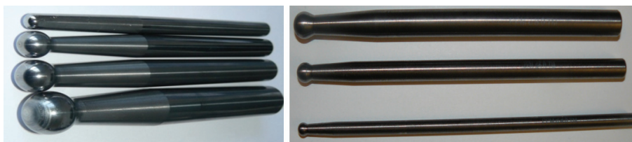
Slika 8.8 Karbidni alati \text{Ø}4 mm, \text{Ø}6 mm (tri alata), \text{Ø}8 mm (dva alata), \text{Ø}12 mm, \text{Ø}16 mm [13, 18]
