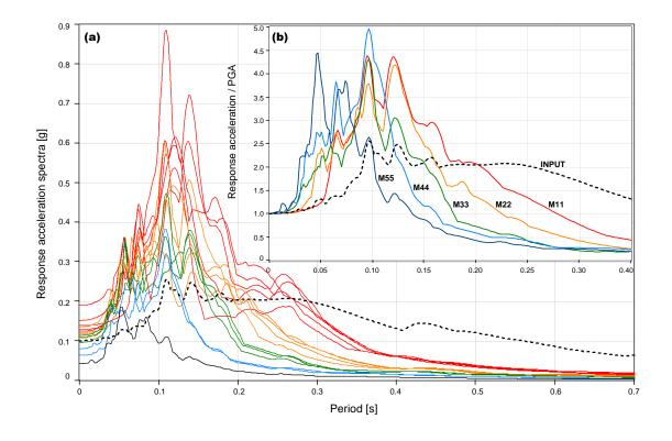
Figure 7.5.: (a) Resultant acceleration spectra for the models with material 1 (red), 2 (yellow), 3 (green), 4 (blue) and 5 (dark blue) as top layer; response spectra of the input accelerogram is represented with a dashed black line and (b) Normalised response spectra for the models with equal upper and lower materials and the response spectra of the input accelerogram.
