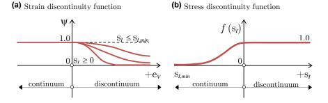
Figure 4.9.: Microplane discontinuity function: (a) strain and (b) stress discontinuity function.
