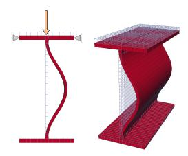
**Figure 3.1.:** Web buckling of a steel I profile.
