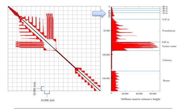
Figure 6.3.: The stifnness matrix topology and its condensed vector form
