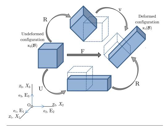
Figure 3.4.: Representation of the polar decomposition of the deformation gradient.
