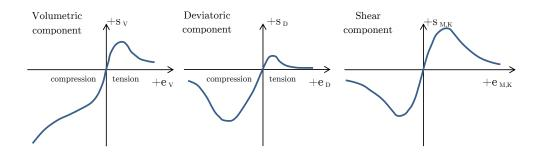
**Figure 4.10.:** Schematic representation of microplane stress-strains relationships for virgin load: volumetric V, deviatoric D and shear-stress components M and K.
