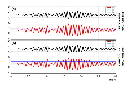
Figure B1.: Reactions of the RC frame columns.
