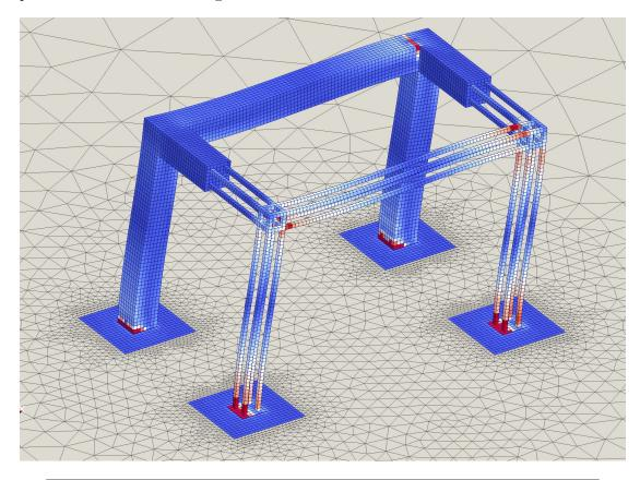
Figure 7.9.: Failure mode of the RC frame.
