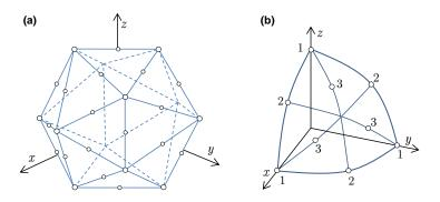
**Figure 4.6.:** Spatial discretisation of the surface of the sphere by 21 integration points: (a) 9th degree without fully symmetric formula and, (b) 9th degree with fully symmetric formula.
