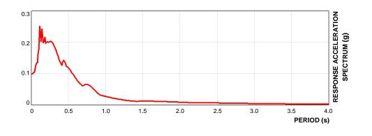
${\bf Figure} \ \, {\bf A3.:} \ \, {\bf Acceleration} \ \, {\bf response} \ \, {\bf spectrum} \ \, {\bf of} \ \, {\bf the} \ \, {\bf used} \ \, {\bf record}.$
