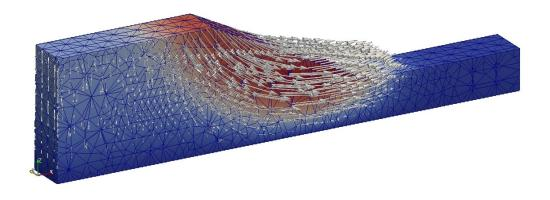
Figure 4.5.: Modelling of a slope failure using the Drucker-Prager yield criterion.
