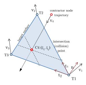
Figure 5.4.: Local detection of contact
