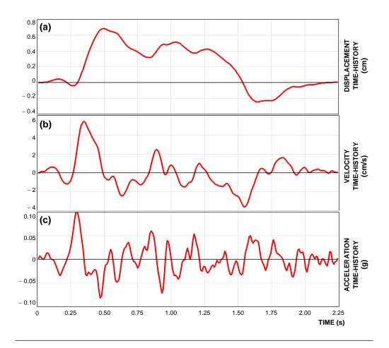
Figure A2.: Displacement, velocity and acceleration time-history of the used record.
