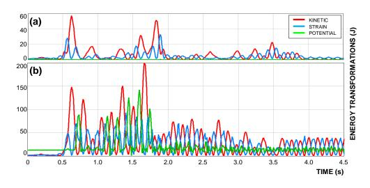
**Figure 7.13.:** Structure energy transformations for PGA = 0.2g and  $\mu = 0.1$  (a) and  $\mu = 0.4$  (b).
