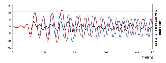
**Figure 7.12.:** Relative displacements for PGA of 0.2g and  $\mu = 0.10$  (black),  $\mu = 0.25$  (blue) and  $\mu = 0.40$  (red).
