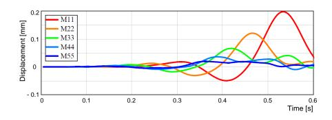
**Figure 7.4.:** Arrival of shear waves at the ground surface (showing horizontal displacements).
