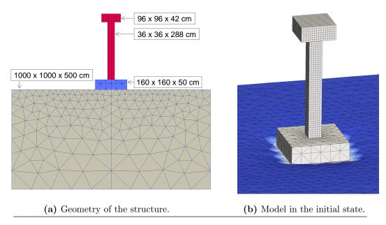
Figure 7.10.: 3D FE model of the structure in the second study
