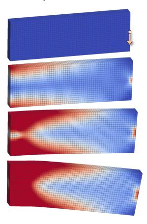
**Figure 4.4.:** Forming of a plastic hinge in a cantilever beam using the von Mises yield criterion.
