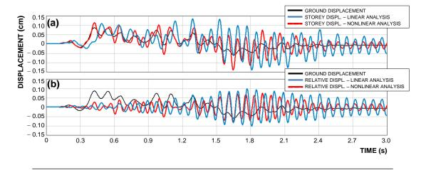
Figure 7.8.: (a) ground and storey and (b) ground and relative displacements for the considered RC frame (model M33) resulting from non-linear and linear analysis with initial stiffness.
