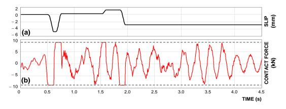
**Figure 7.11.:** (a) horizontal slip between the foundation and the soil and (b) horizontal contact force, both for PGA of 0,2g and  $\mu$  of 0,1.
