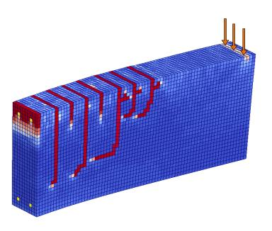
Figure 4.13.: Cracking of a reinforced concrete cantilever beam.
