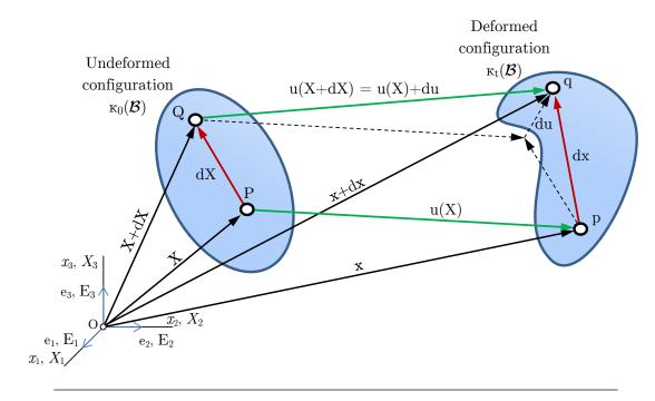
Figure 3.3.: Deformation of a continuum body.
